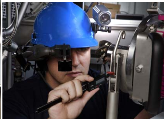
I-BORO® – the mobile service tool with portable mini-PC, safety helmet with zoom camera, control display screen and headset
