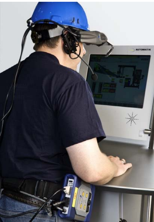
I-BORO® – the mobile service tool with portable mini-PC, safety helmet with zoom camera, control display screen and headset
