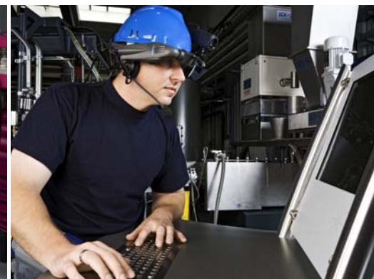
I-BORO® – the mobile service tool with portable mini-PC, safety helmet with zoom camera, control display screen and headset
