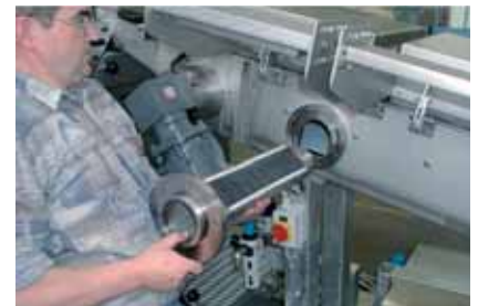
Variable positioning of exhaust air nozzle
