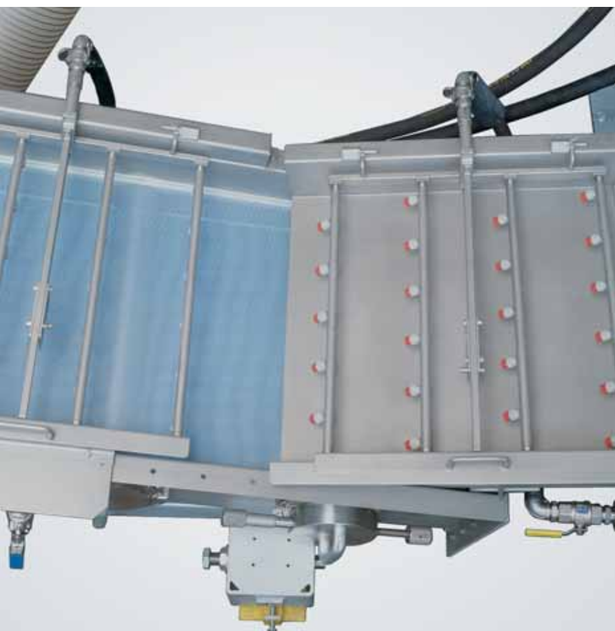
View of the transition zone from strand guide to conveyor belt
