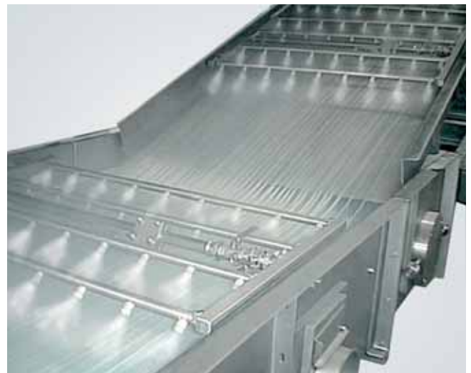
Transition zone from strand guide section to conveyor belt
