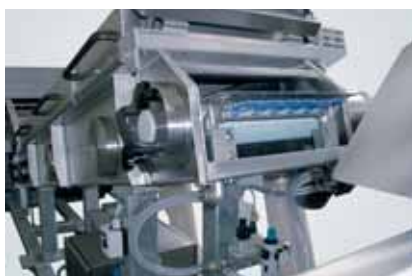
Air nozzles at the transition to the pelletizer
