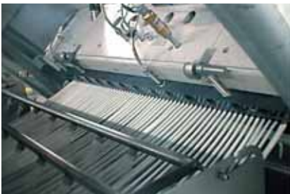
SG 900 die head in operation
