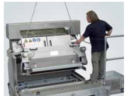
M-USG 1200 V: Quick exchange of cutting head
