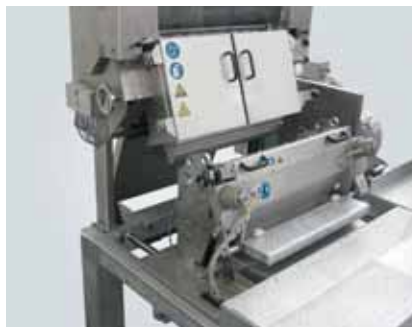
M-USG 900 V: Cutting head in changing position
