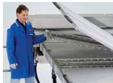
M-USG 1200 H: Strand guide section with spray bars which can be easily removed
