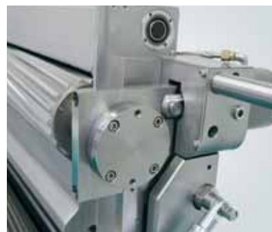
Feed roll bearings outside of the cutting chamber
