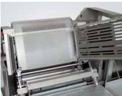
M-USG 1200 V: Strand guide section showing individual strand guide
