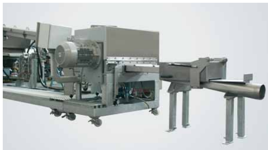
After cooling line with agglomerate separator
