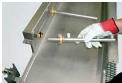
Strand guide section with replaceable spray tubes
