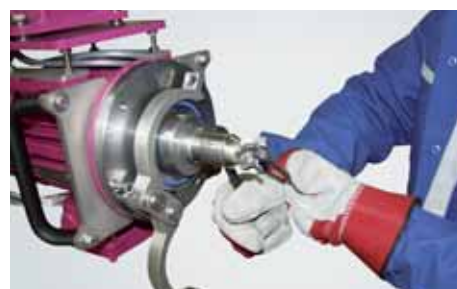
Disassembly of the knife head with minimal hand movements
