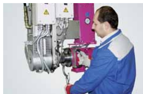
Quick and easy opening of the cutting chamber
