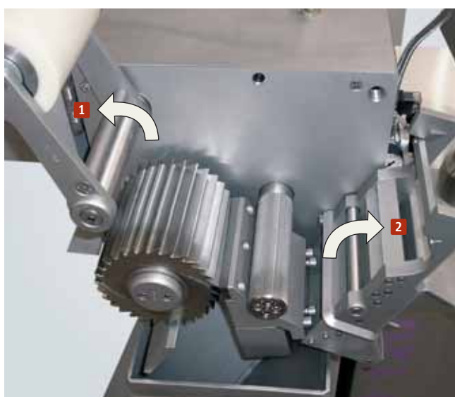
PRIMO E and PRIMO S strand pelletizers: Quick and easy access to all cutting chamber components, without the need for tools
