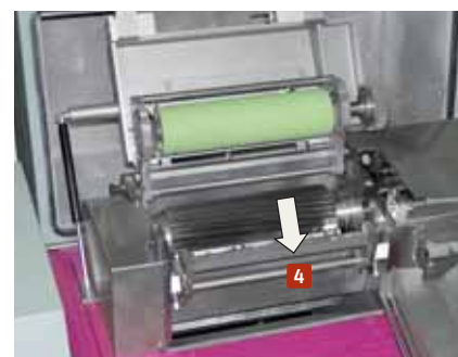
Patented cutting rotor with positive interlock
