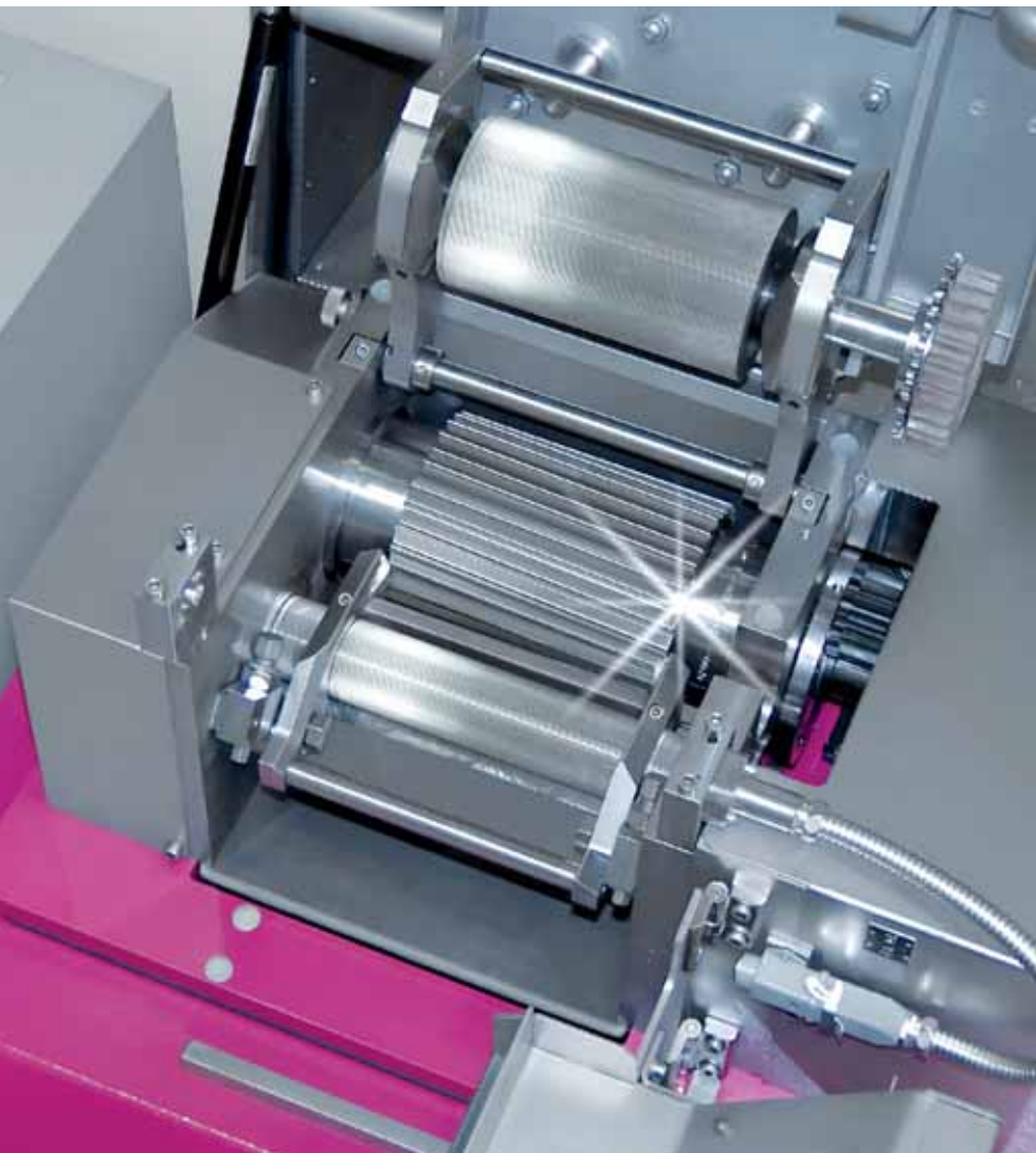
View into cutting head PRIMO Plus 200
