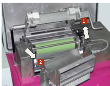
Strand pelletizers PRIMO Plus and M-ASG: Quick access without tools to all cutting chamber components
