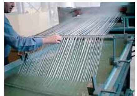
Cooling trough KW 600 for up to 60 strands
