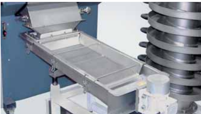
Classifier and spiral conveyor for final pellet treatment
