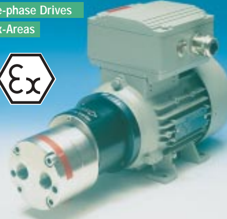
Constant-speed three-phase motor (IP 55, increased safety) for Ex-Areas, degree of protection EEx e II T3, constant speed rates available on request, n = 2,750 rpm, n = 1,350 rpm, n = 900 rpm, 3 x 230/400 V, 50 Hz
