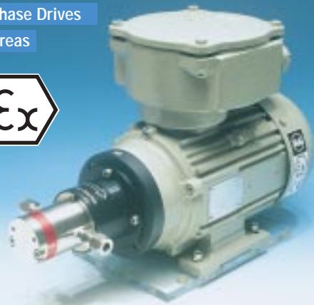
Three-phase motor (IP 55, flame-proof enclosure) for Ex-areas, degree of protection EEx de IIC T4, controlled via frequency converter, n = 200 - 6,000 rpm, external control capability, 1 x 230 V, 50/60 Hz
