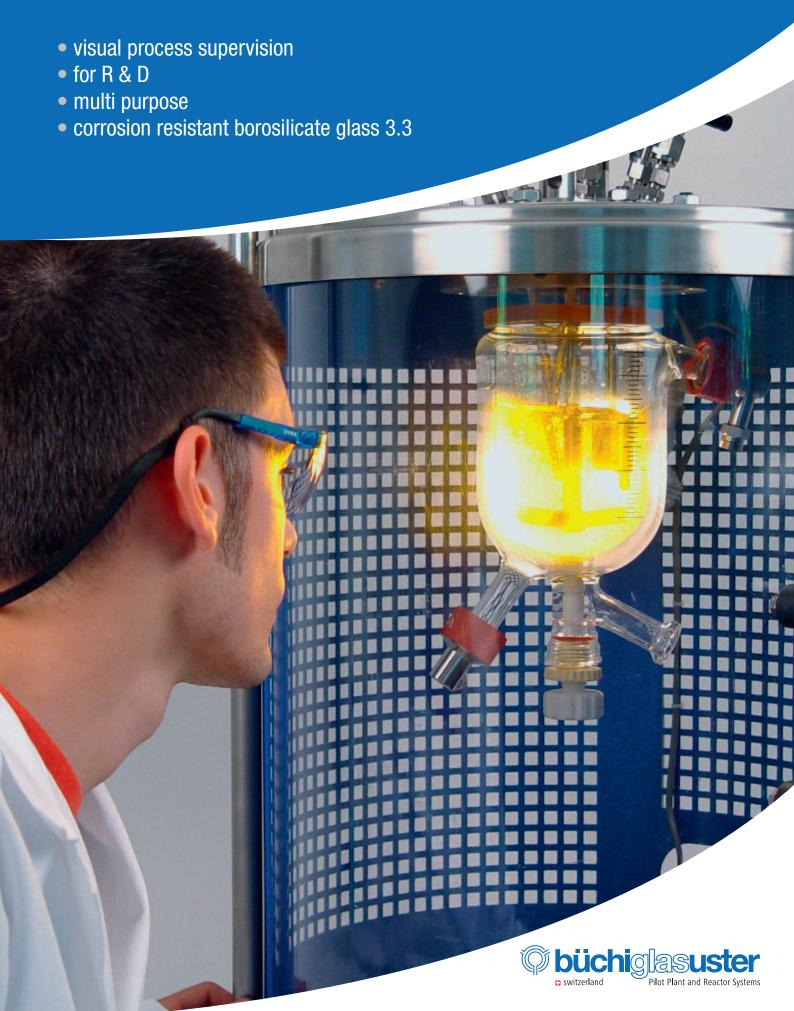
Büchi carries a complete range of pressure autoclaves with glass vessels. Our program includes jacketed glass vessels from 100ml up to 5 liter with maximum operating pressure up to 12 bar, depending on the vessel size. Some systems can also be equipped with steel vessels for operation up to 60 bar.
